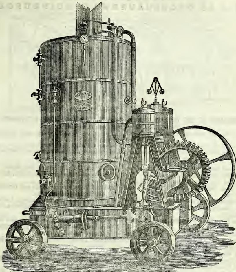
THE 'FIELD' BOILER, AND ENGINE ATTACHED.
