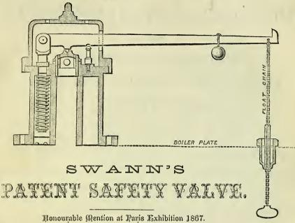
This Valve is the ordinary Steam Valve, until undue weight is applied, when it becomes a Safety Valve. Firemen are unable to tamper with this Valve, either with Steam off or on. Indicates Deficiency of Water in Boiler. The Insecurity to Life and Destruction to Property arising from Over-Pressure or Deficiency of Water are completely Guarded Against. No Steam-Boiler should be without it.
