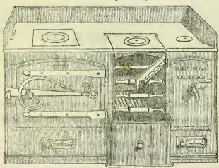
Extra Strong Close Range, as Drawing, with Oven and Boiler and Skirting Plates, 42 in., £5, 15s.;
