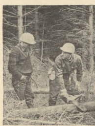
A tool instructor shows a forest worker the right way to use a power saw for felling, that is, trimming off side branches, from a felled spruce tree. Both wear protective helmets.
