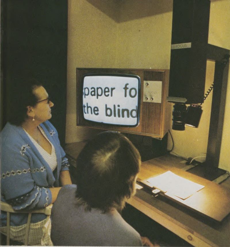
A close-circuit television system that magnifies objects placed beneath a camera lens as an aid for the partially sighted.
