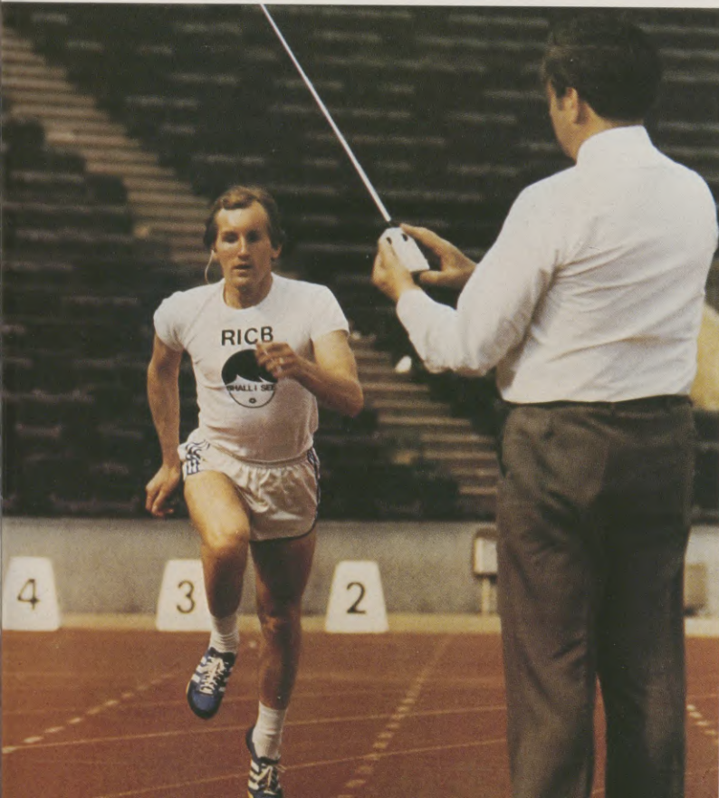
An audible aid to guide blind athletes has been developed by the founder of the charity Research into Child Blindness. The inexpensive, completely portable, system emits a high or low bleep which is transmitted to the earpiece worn by the athlete.
