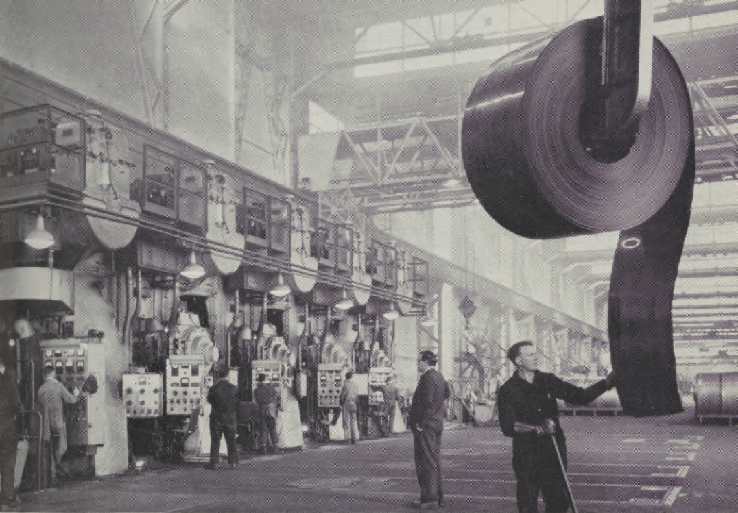
The Trostre tinplate works of the Steel Company of Wales. Coils on a rack await cold reduction at the 5-stand mill while an overhead crane removes a cold-reduced coil.
