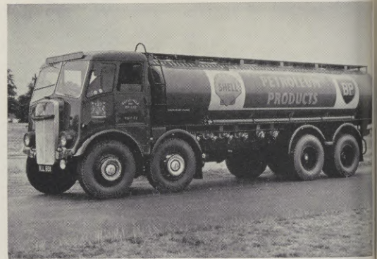
Motor spirit road tanker with a capacity of 3,600 gallons.
