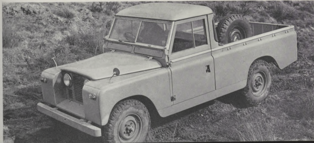
The 1958 Land-Rover 109 , with 4-wheel drive and 2½ litre engine. In ten years more than 200,000 of these multi-purpose, cross-country vehicles have been manufactured, about three-quarters of them for overseas.
