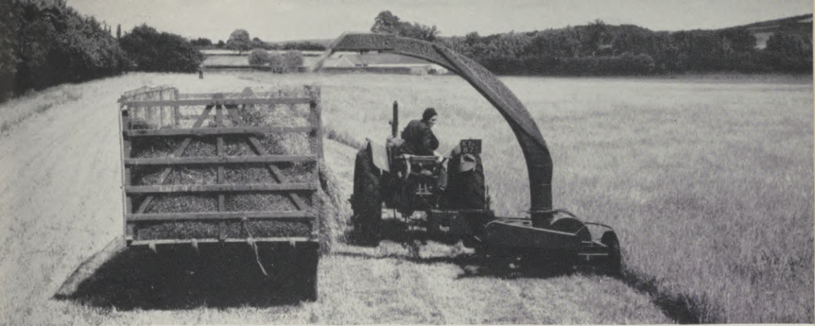
The Hayter silorator harvester lacerates the grass so that the cell tissue speedily ferments.
