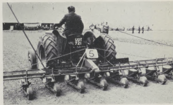
Precision seed drills save seed and labour: this Stanhay drill is power-driven.
