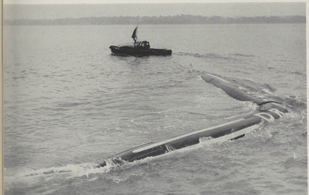
The Dracone flexible barge (see p. 206) can be folded for transportation when empty.
