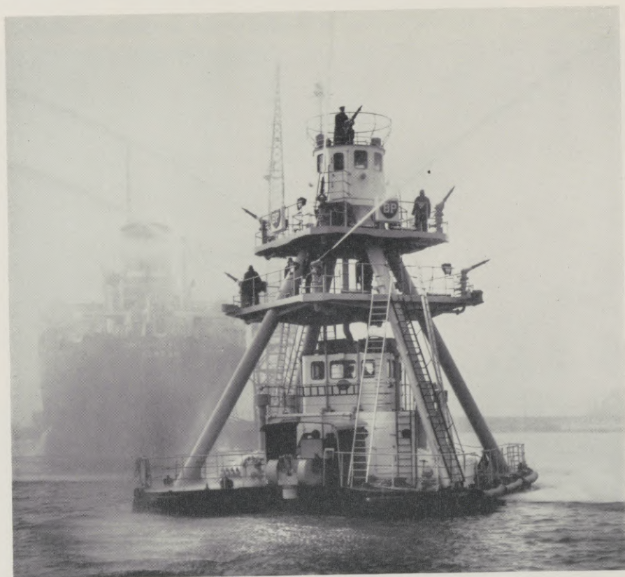
The Firemaster , a new type of fire-fighting float, with 40-foot tower, designed by the BP Tanker Company for use in Swansea Harbour, South Wales.
