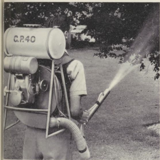
A new chemical spray powered by a two-stroke engine.
