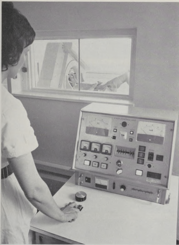
Left: Computerized scanner for diagnosing brain diseases gives 100 times more information than conventional X-ray methods.
