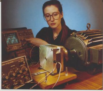
At the National Engineering Laboratory, East Kilbride, Scotland, engineers have designed and built a suite of wire rope testing machines, enabling them to assess accurately the performance of the large-diameter wire ropes used for anchoring structures in the offshore oil industry.
