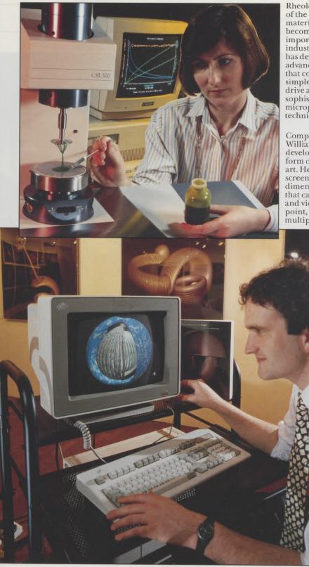
Rheology, the study of the viscosity of materials, has become increasingly important in many industries. Carri-med has developed an advanced rheometer that combines a simple mechanical drive and highly sophisticated microprocessor techniques.
