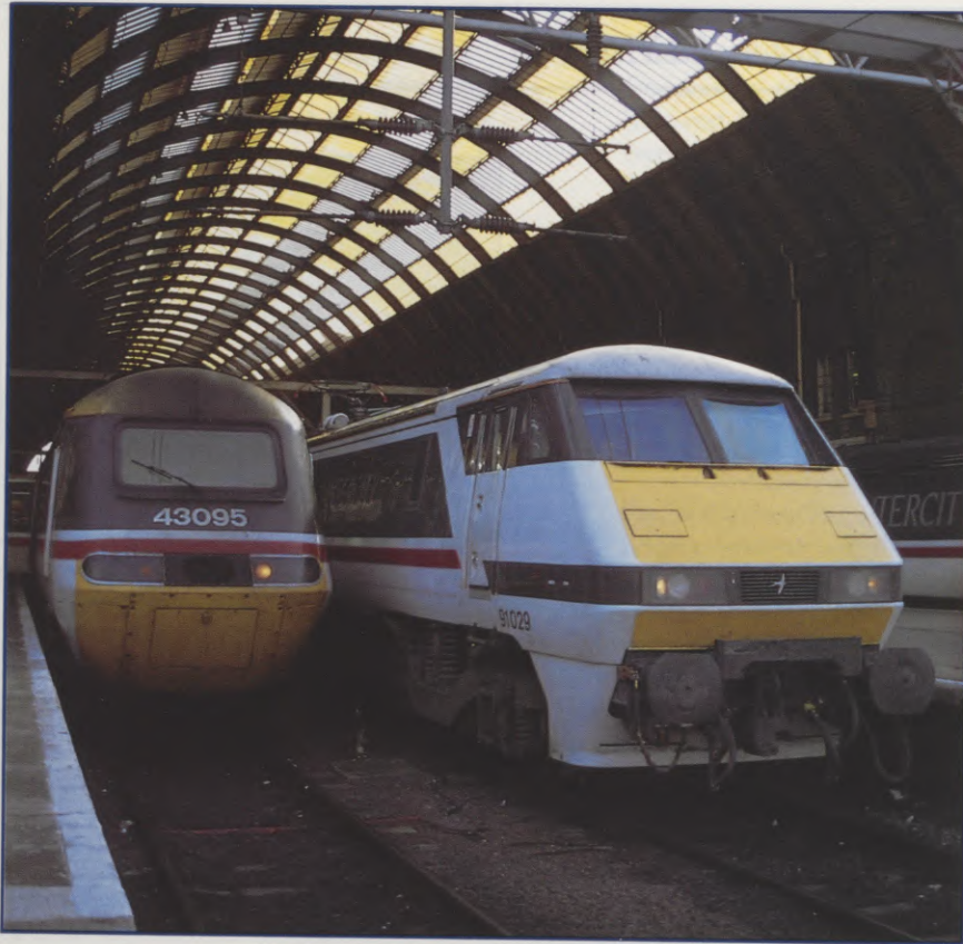
British Rail's new InterCity 225 trains have been introduced on the recently electrified London-Edinburgh east coast main line. The InterCity 225, seen on the right of this picture, is designed to travel at speeds of 225 km/h.
