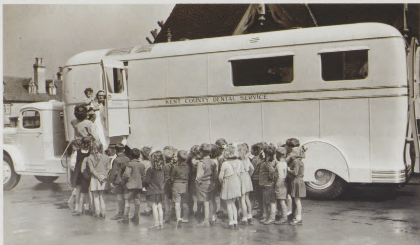
Children at Aylesford, Kent, visit a mobile clinic in 1949. It had a waiting room for six people, a surgery and a combined recovery room and laboratory.
