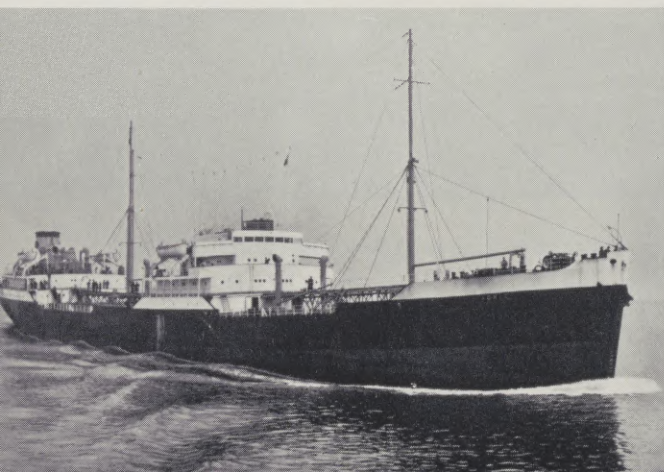
The world's first merchant ship to be powered by a gas turbine engine: the tanker Auris .
