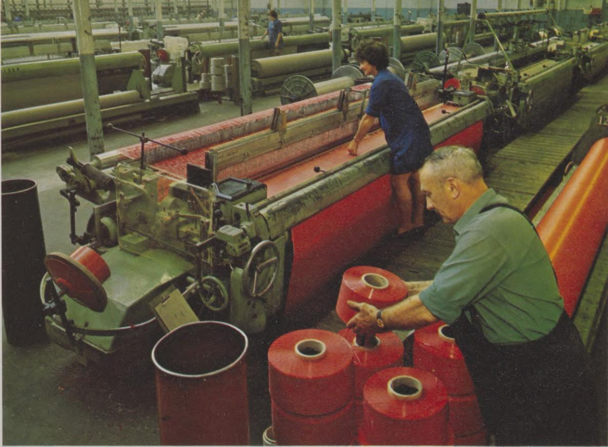
Weaving polypropylene fabric on looms in a former jute factory at Dundee, Scotland.
