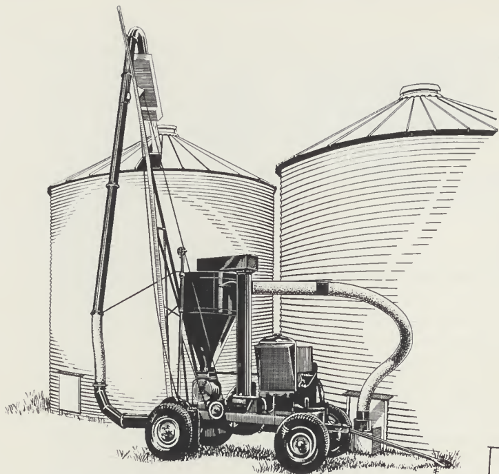
Fig. 3 Mobile pneumatic elevator
