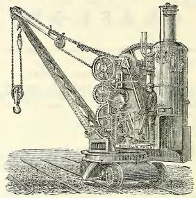
14-TON LOCOMOTIVE STEAM CRANE AT PARKHEAD STEEL WORKS, CLASCOW.
