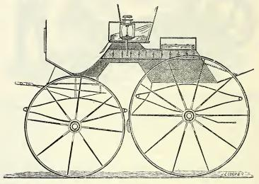
A LSO Maker of the Zetta (or Two-wheeled Brougham), a complete Open or Close Machine the Carriage parts being fitted in such a manner that the Balancing of the Machine entirely subject to the Driver's control, and, with the assistance of the Brake, not only reta the progress of the Machine when descending hills, but removes the weight from the horse's ba P. H. having had long practical experience in America and this country, is better enabled execute all Orders intrusted to him.
