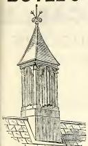
Effectually extract the foul air, have no mechanical motion, are entirely free from down-draught, and can be constructed to har monize with every style of architecture.
