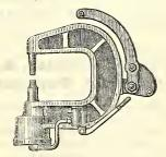
Patent Hydraulic Boiler Riveting and Flanging Machines. Patent Hydraulic Portable iveting Machines for Ship, Bridge, and Boiler Work. With our Patent arrangement of Duplex Minks, our Riveting Machines give the same Pressure on the Rivets as other Machines, with a living of 75 per cent. of Pumping and Accumulator Power.
